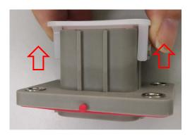
两边均匀用力取出防尘 盖备用 Remove the dust cover with even force on both sides
