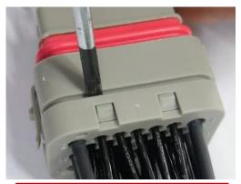
用镊子或螺丝刀将卡位翘起 Use tweezers or thin screw driver to pry up the back cover Buckle position
